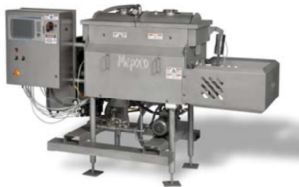
Model TB170-0075 – ThermaBlend batch cooker @ 75 Gal (single agitator)
