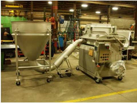
Mepaco 420v stuffer with inter-connecting piping and round jacketed hopper.
