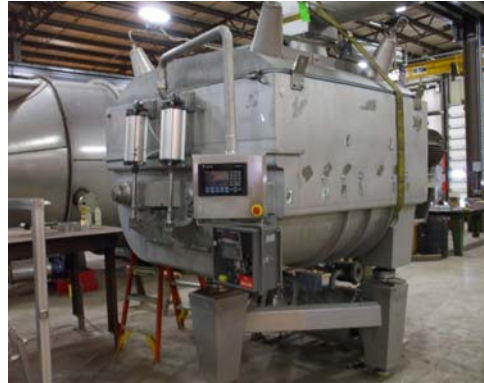
R-1258: 3500# Wolfking UNI-Mix vacuum mixer, paddle agitators, complete controls with touch screen, vacuum pump, Emery load cell system and CO2 snow horns.
