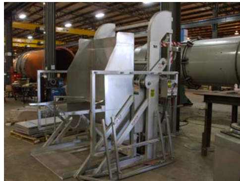
R-1259: Mepaco 519 vat dumper with power pack, controls, juice catcher and accommodate v-mag buggy arms.
