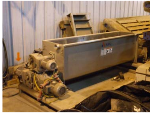
116322: 1200# dual 9" auger cart w/16" leveling ribbon and new 20 Hp Fristam 250 pump.
