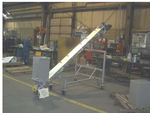
5203---Mepaco Model 185-1 incline screw conveyor—6” with a 65” discharge height, complete with VFD controls.
