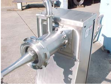
Model 6-61L (160mm) inline "rework" Grinder @ 15 HP.
