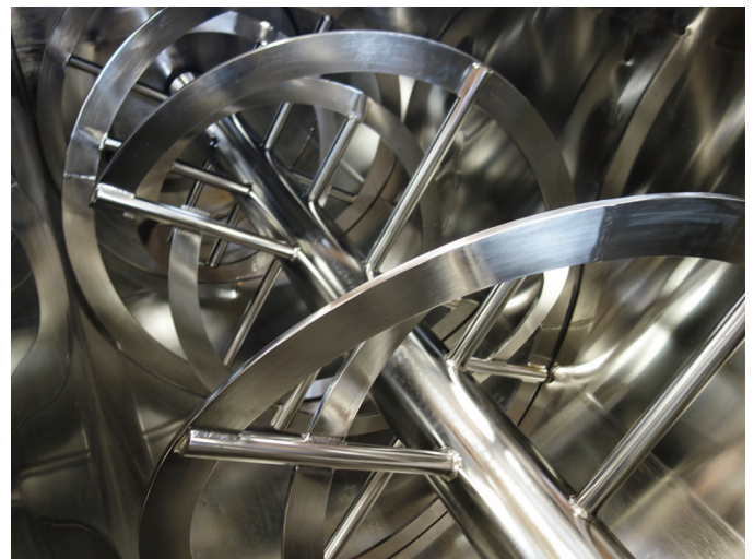
A single shaft with dual ribbon agitator is shown inside an industrial cooker with electropolished finishes
