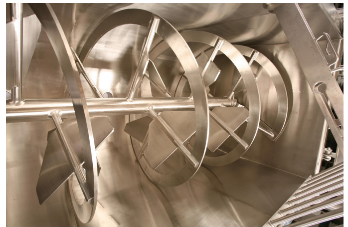
Single Agitator with Ribbon /Paddle Flights
