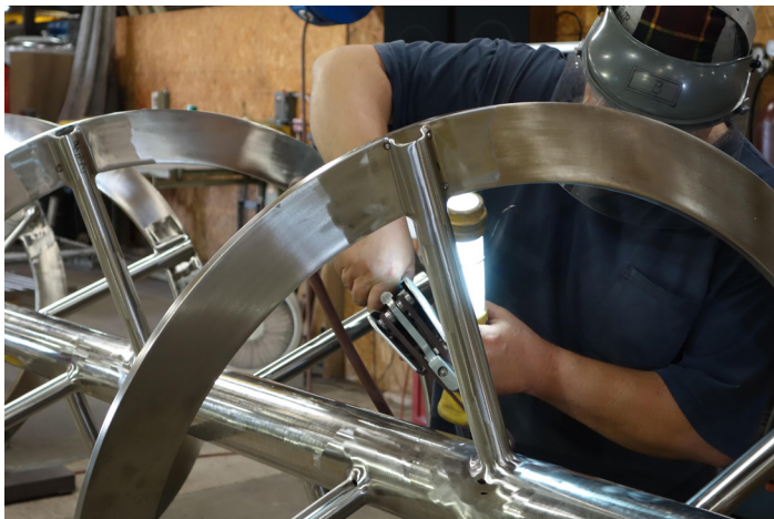
One of Mepaco's fabricators putting finishing touches on a leveling ribbon
