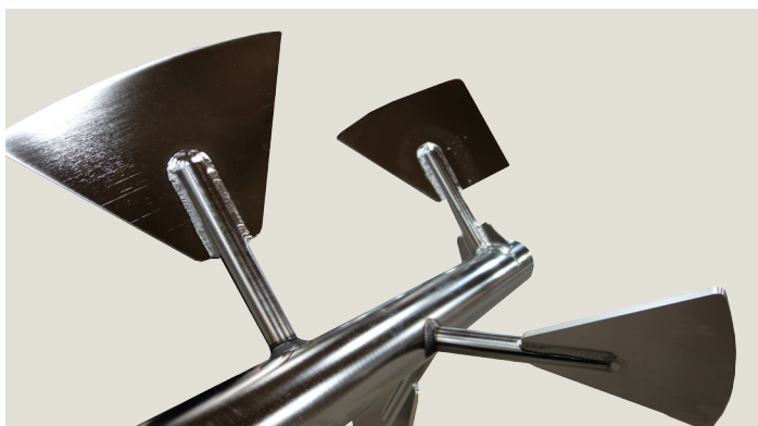
In production, this single shaft paddle agitator is staged for electropolishing before being installed in an 8000 lb. mixer.
