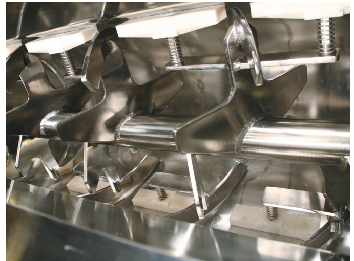
Single shaft agitator with dual paddle flights showing scraper system
