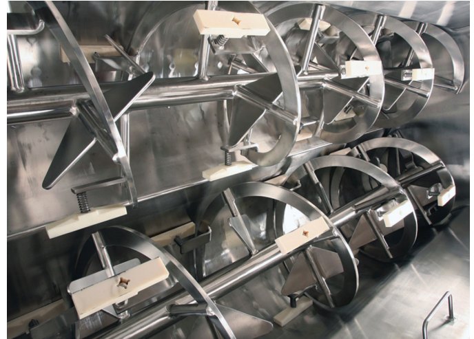
Single Agitator with Ribbon /Paddle Flights
