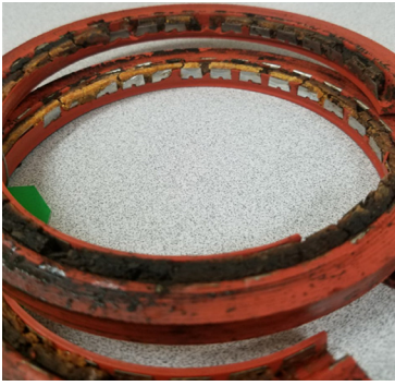
Worn and broken seal
