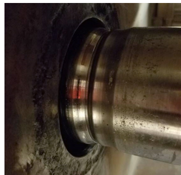
Excessive wear resulting in grooves on shaft caused by worn mechanical seal.
