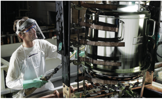
A portable vessel used in the pharmaceutical manufacturing industry emerges from the electropolishing tank at Apache Stainless Equipment Corporation.
