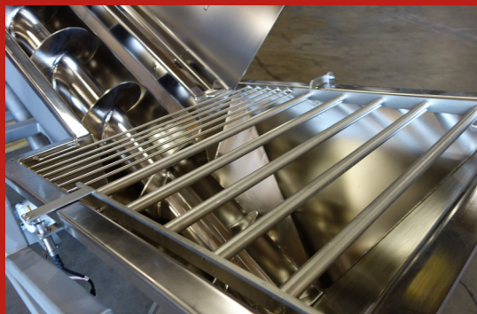
Electropolished food contact surface with magnetic grate
