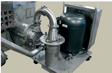
Vacuum Stuffer with Emulsifier
