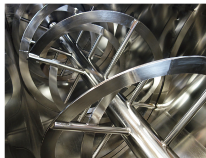
◀ A single shaft with dual ribbon agitator is shown inside an industrial cooker with electropolished finishes
