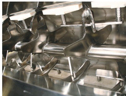
Single shaft agitator with dual paddle flights showing scraper system
