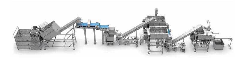
Pre-Blending offers a seamless, accurate solution, but the equipment costs, added footprint size, maintenance, and sanitation requirements must also be considered. In this method, lean and fat are transferred into one of two pre-blenders. The goal is to create a homogeneous batch of each lean point (preground) from which the final mixer can draw.
