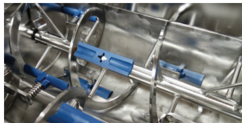
Patented, metal detectable scraper system showing coil spring design
