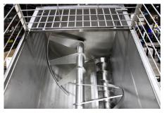
The Clean Sweep Surge Loader has been engineered for prepared foods, ground, or trim meat products. The design is modified to meet the requirements of the application, including:
