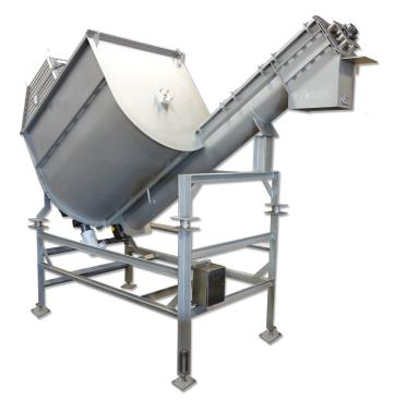
Integral to the Bin Batching System are the Metering Screw Conveyors, designed with a Clean- Sweep hopper. The Clean-Sweep hopper offers a solution that mechanically clears food product between batches on metering or surge loading applications. The ribbon agitator gently and continually pushes product into the feed screw.
