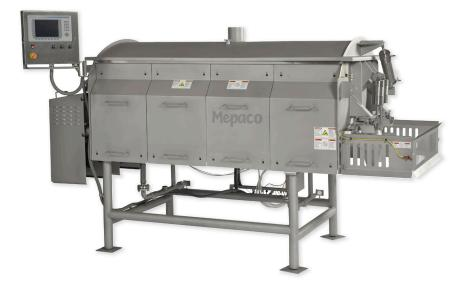
In the system, the food processor required a versatile cooking solution to efficiently blend and cook various soups and sauces, all with different process recipes and controls. The ThermaBlend® was specified for the "Dual Cook System" because of its ability to blend and cook the processor's viscous products with superior efficiency.
